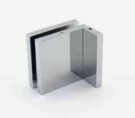
Morsetto quadro 50x50 mm vetro-muro - vetro 6-8-10 mm Glass-wall square clamp 50x50 mm - 6-8-10 mm glass
