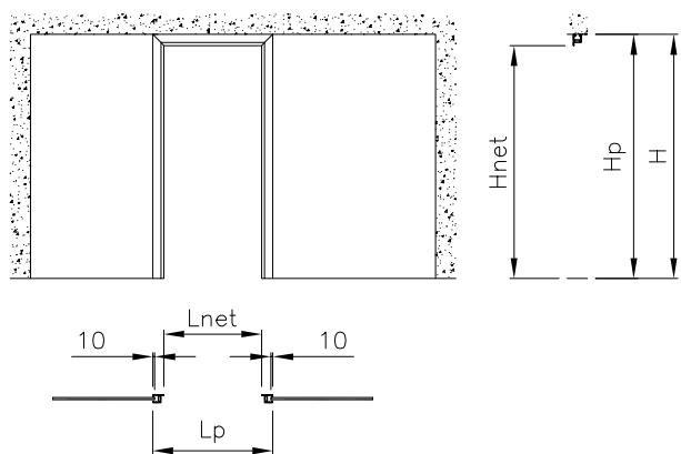
$$L_{net} = \max 1090 \text{ mm (C7-C8)} \max 1790 \text{ mm (C7D-C8D)}$$
