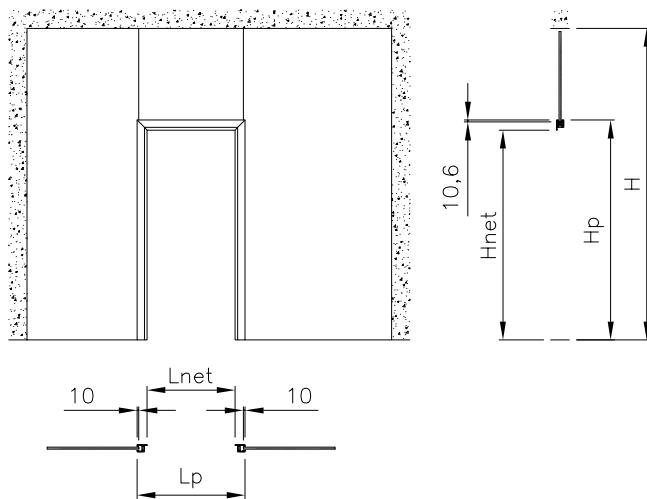
$$L_{net} = \text{max } 1090 \text{ mm (C9) max } 1790 \text{ mm (C9D)}$$
