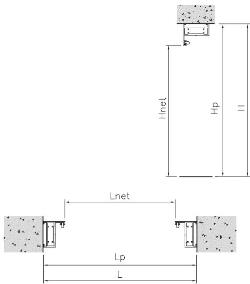
$$L = \text{max } 1200\text{mm (C1-C2)} - 1900\text{ mm (C1D-C2D)}$$
