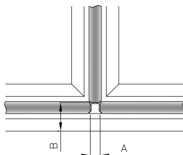
con vetro da 10 a 10,76 mm/with glass from 10 to 10.76 mm A = 9 mm B = 24 mm
