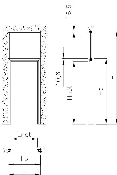
$$L = \text{max } 1200 \text{ mm (C3)} - 1900 \text{ mm (C3D)}$$
