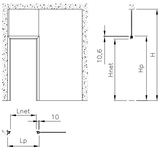
$$L_{net} = \max 1090 \text{ mm (C6)} \max 1790 \text{ mm (C6D)}$$
