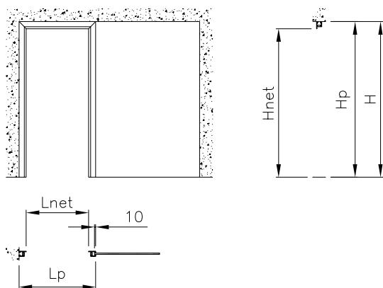
$$L_{\text{net}} = \text{max } 1090 \text{ mm (C4-C5) max } 1790 \text{ mm (C4D-C5D)}$$
