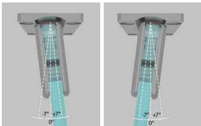
All adjustments can be done when the door has already been installed. No need to disassemble any hinge component
