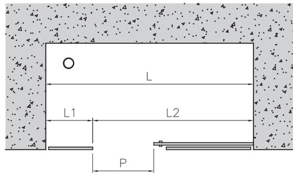
con/with  $B1 \neq B2$      $L1 = L - L2$      $B1 = L1 - X1$
