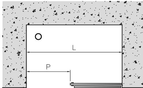
$$L = da/\text{from } 840 \text{ a/to } 2200 \text{ mm}$$
