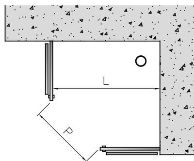
$$L = da/\text{from } 875 \text{ a/to } 975 \text{ mm}$$
